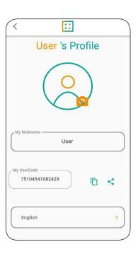
The User sends his own UserCode to the installer. The Installer memorizes and enables it (consuming a mobile credential). The User, than, has just to connect to the receiver, the app will do the rest. If the Smartphone is memorized and correctly enabled, it will be created a button. The User can personalize it changing the icon or the name.
